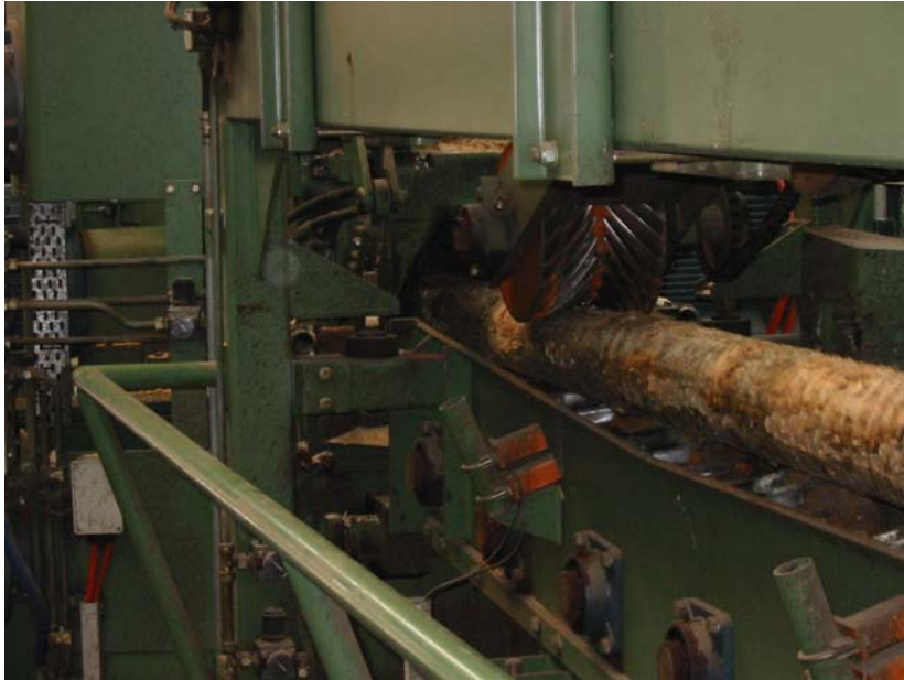
Figure 4-3: Log entering Hew Saw
